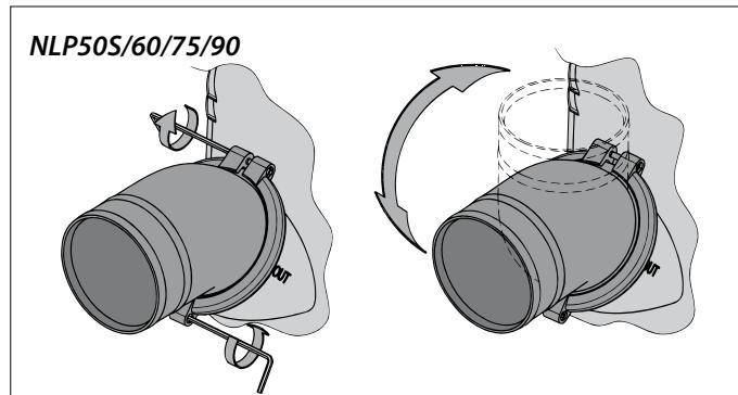
In order to achieve the ideal connection between the hoses and the waterlock, both hose connections turn through 360 degrees.
