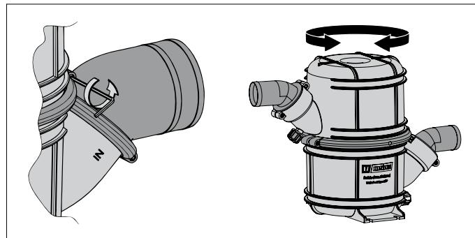
The top portion of the waterlock can be turned in a 360° radius.
