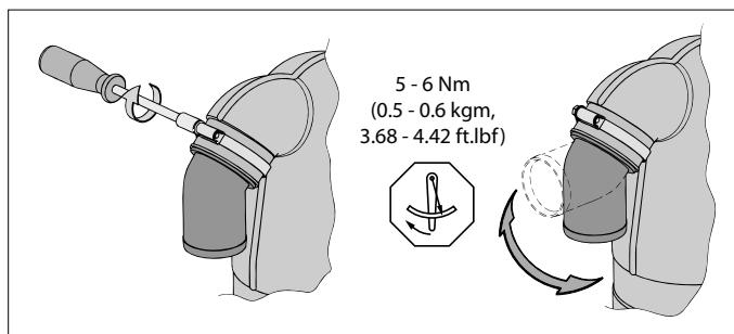
**LGS 60, 75, 90:****Unscrew the hose clamps before turning the hose connections!**Re-tighten the hose connections with a tightening torque of **0.4 Nm (0.3 ft.lb)**
